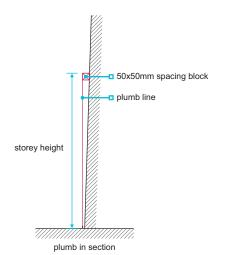
Example: Using 50mm wide spacing blocks, the plumb bob should be 42-58mm from the wall, measured at between 2.5-3m from the spacing block.
