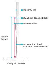
Example: Using 25mm wide spacing blocks, the masonry line should be 17-33mm from the reference line
