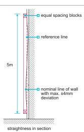
Example: Using 25mm wide spacing blocks, the masonry line should be 21-29mm from the reference line.
